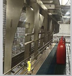
Combination of mechanical and pneumatic driven product marshalling infeed systems.
